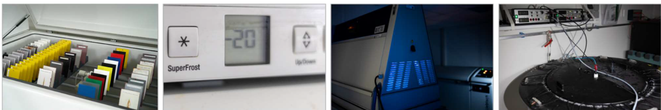
Figure 3: test equipment: salt spray, freezer, UV/condensation cabinet and cathodic protection set-up
